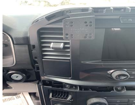
InDash installed showing location
