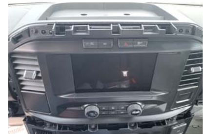
Front of display screw location
